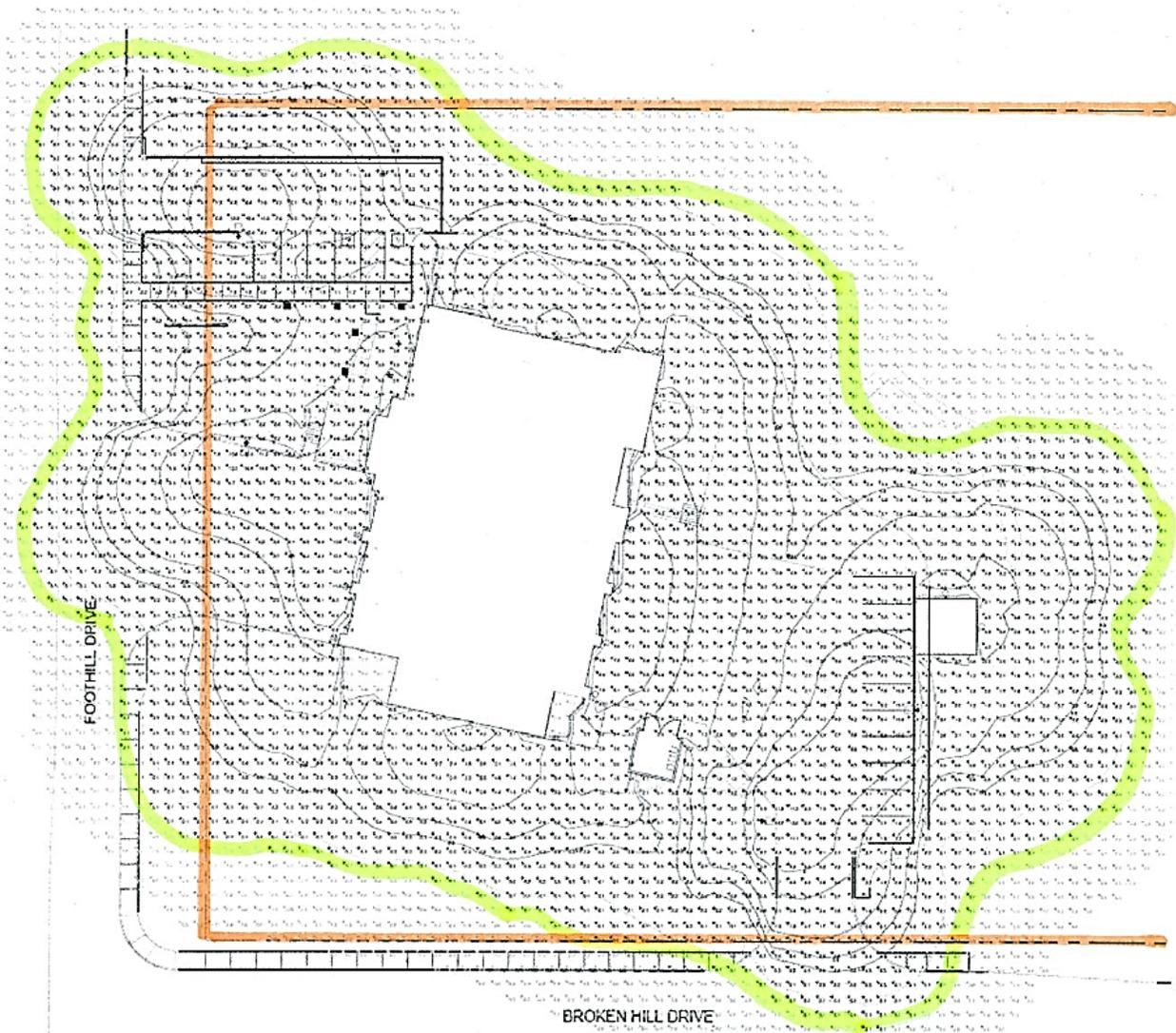
The applicant later submitted the following, revised, photometric plans which show compliance with the requirements of the Development Code. This revised plan will be required for approval of building permits. Again, the property line is shown in orange and the lit areas in green.
